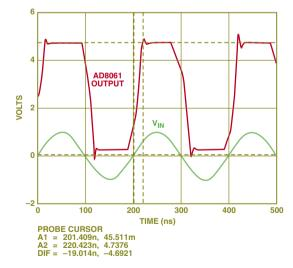
Figure 7. Response of AD8061 as a zero-crossing comparator.
