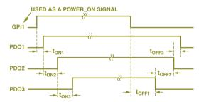
Figure 4. Controlled power on/off sequence using the ADM1060.
