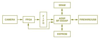
Figure 4. Block diagram of the processing board.
