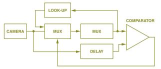
Figure 7. Simplified signal flow diagram of the 1D AR.
