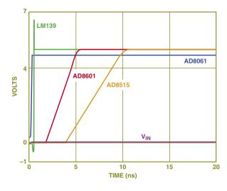
Figure 8. Step response of three amplifiers and a popular comparator. Note the especially fast response of the AD8061.
