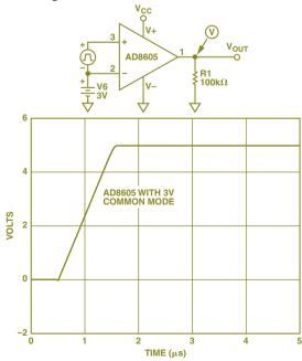
Figure 2. Response of open-loop AD8605 to a 100-mV differential step with 3-V common-mode voltage. Note the essentially linear slewing between the 0- and 5-V rails, and the clean saturation.
