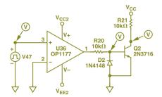
Figure 9. OP1177 connected for comparator operation, with translation and protective circuitry for TTL output.
