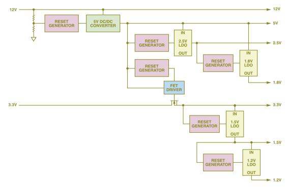
Figure 1. Discrete implementation for sequencing seven supplies.
