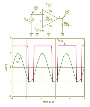
Figure 3. Response of an OP777 amplifier to a  $\pm$ 2-V, 1-kHz signal, biased by +2V, and compared with a +0.5-V dc level. Note that there is no phase inversion for this large swing. However, the gain is quite low at a common-mode level of +0.5 V from the negative rail, as can be seen by the approximately 0.3-V overdrive that is needed.
