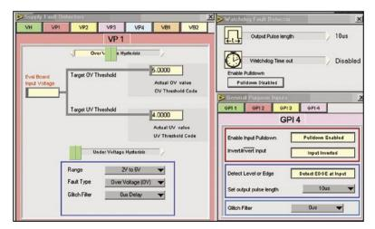
Figure 2. ADM1060 graphical user interface (GUI).
