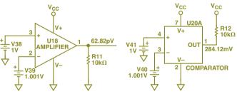
Figure 1. Responses of single-supply amplifier (63 pV) and comparator (280 mV) models to a -1-mV input-voltage difference.
