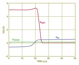
Figure 10. Response waveforms for the OP1177 comparator circuit.
